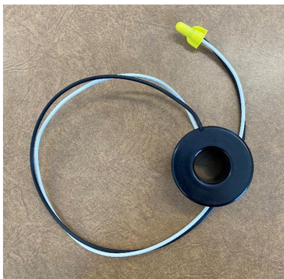
Current transformer – supplied by SCEC
